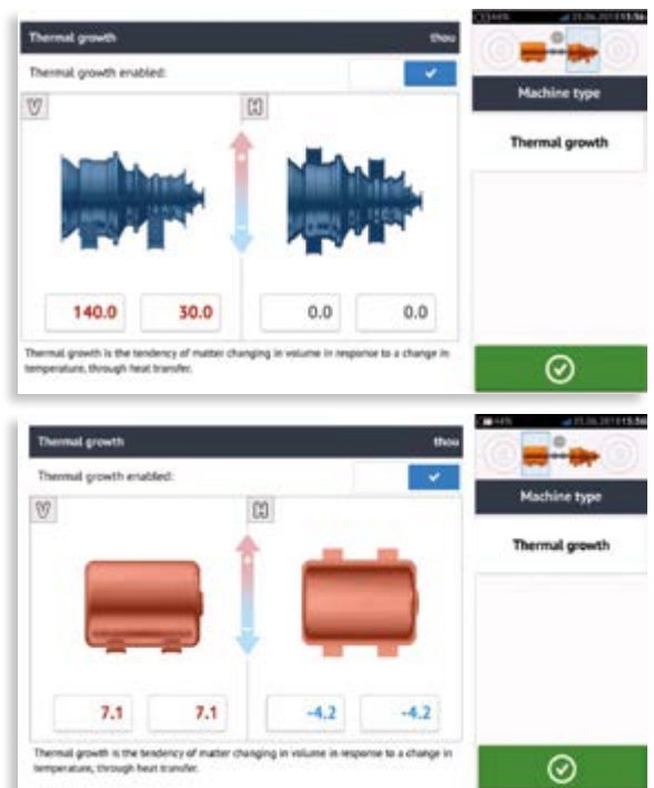
Fig 6: Thermal Growth Allowances
